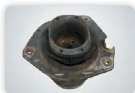
Torn Strut Insulator
