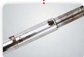
Damaged piston rod
