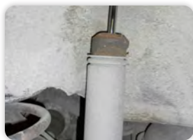
Loose bump stop
